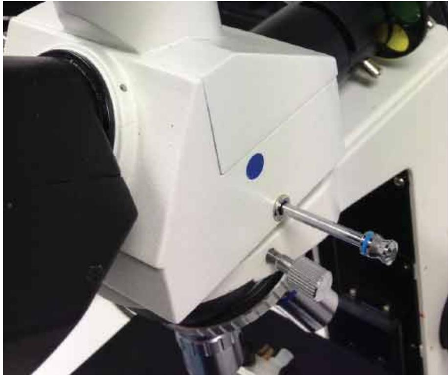
Image 1. LM10 filter position. The fluorescence filter is fitted on the right hand side of the microscope optical head (see red arrow). The colored dot indicates that the filter has been fitted. To insert the fluorescence filter, the silver lever must be pushed in.
