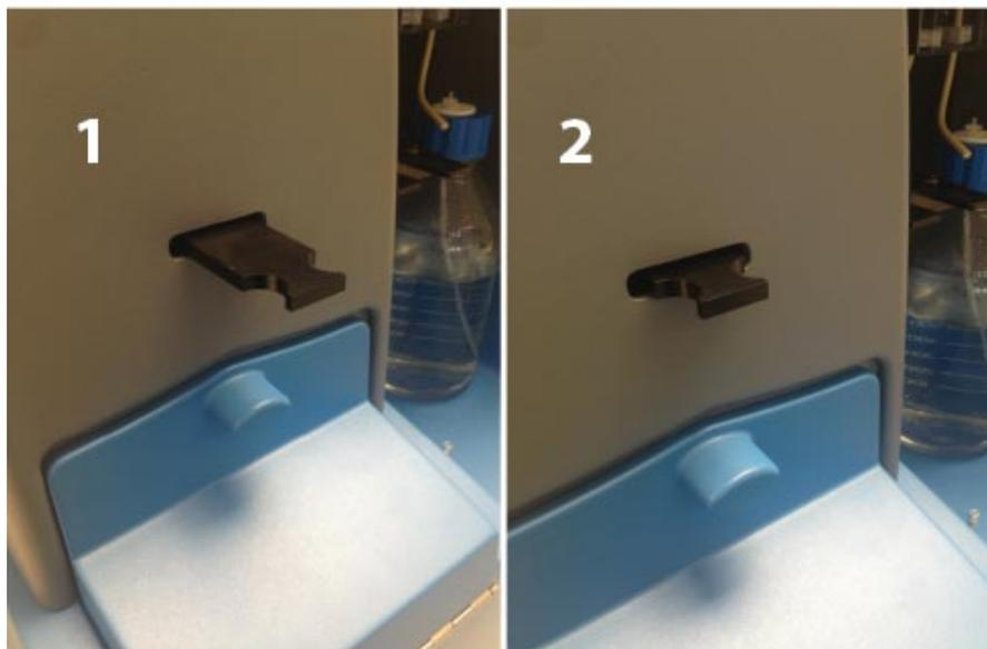
Image 2. (Top) The NS500 filter holder. The colored dot shows the position of the fluorescence filter. (Bottom) Position 1 - the clear glass filter is inserted - this position should be used for light scatter mode. Position 2 - the fluorescence filter is inserted - this position should be used for fluorescence mode. These positions are correct if the fluorescence filter is fitted as shown in the top image.
